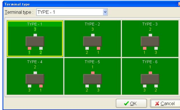
[Fig.143] Terminal type (Mini-module-3 (TYPE1))
