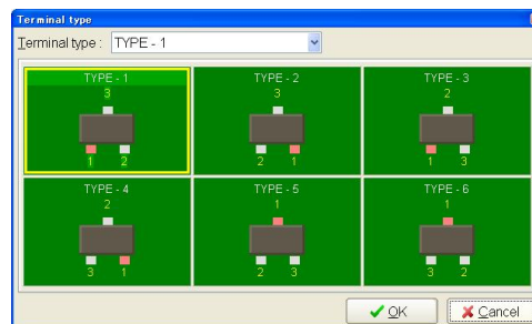
[Fig.149] Terminal type (Mini-module-3 (TYPE1))
